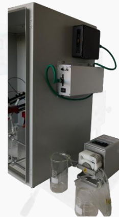
View on right side of Faraday cage with computer and dispensing peristaltic pump
